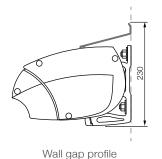
Optional extruded profile used to flash the cassette of the awning to the wall.
